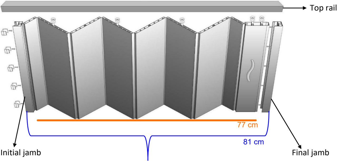
After installed, the width is 81cm (from Initial jamb to Final jamb) when folding door is closed. Top rail we provided is 81cm too.
