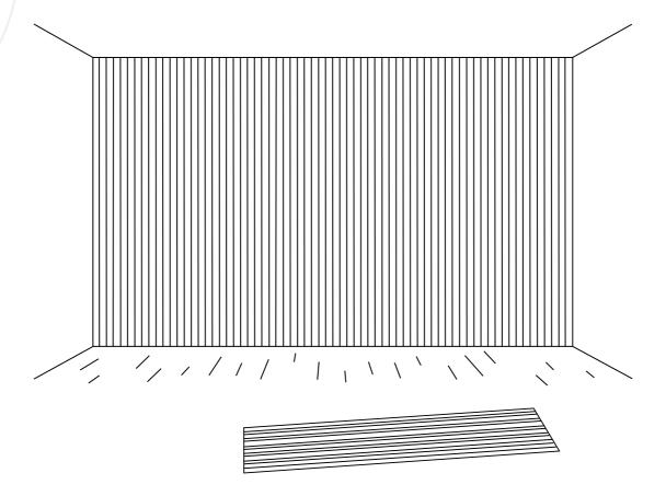
To mount the acoustic panels, add them to the wall and screw the 35 mm black screws into the felt at the same height as your battens (or with a distance of 60 cm if applied directly).
