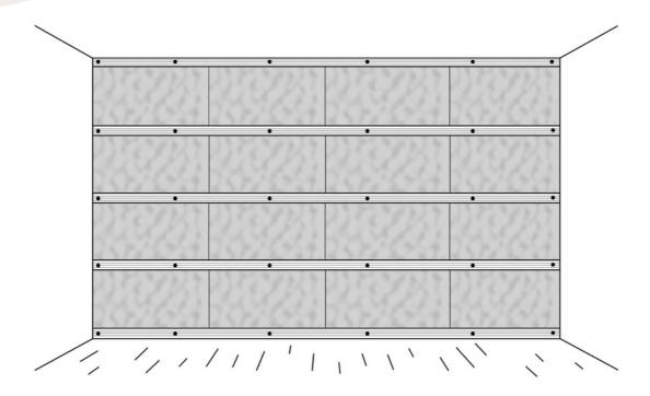
Apply the 45 mm mineral wool between the battens to achieve the best possible acoustics. The mineral wool can be cut using a box cutter to fit just right.
