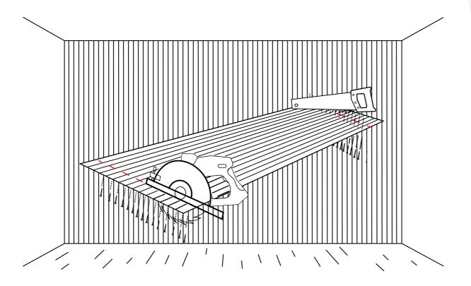
If the panels are too tall, you can also saw some of the height off. Start by using a pencil to mark a line where you want to cut.
