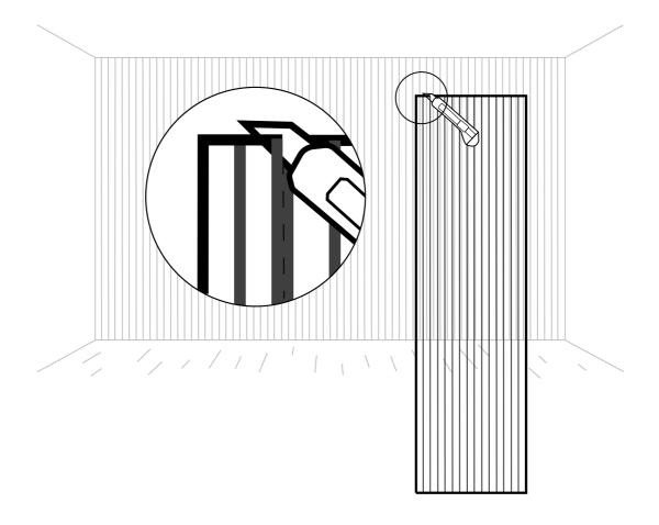
Cutting the width is super easy. First, you measure where you want to cut. Then you have to use a sharp knife (like a box cutter) to cut a line in the felt.
