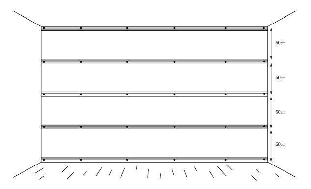
We recommend using battens and mineral wool behind your Nordic Acoustic panels. The reason is that this creates the highest sound absorption possible (known as Sound Class A).
