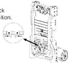
10. Pull handle up to retract wheels and lock in place.
