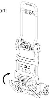
8. Press the levers to unlock and fold handle down.
