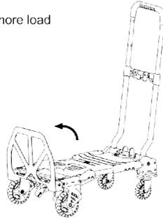
6. Press levers to unlock, lift handle up for 2 wheel cart usage.
