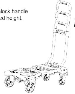
5. Lift the base plate if more load control is desired.
