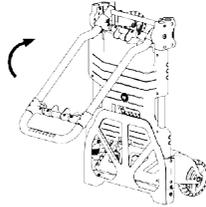
4. Press levers to unlock handle and raise to desired height.
