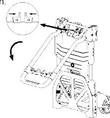
9. Press levers and lock handle in folded position.
