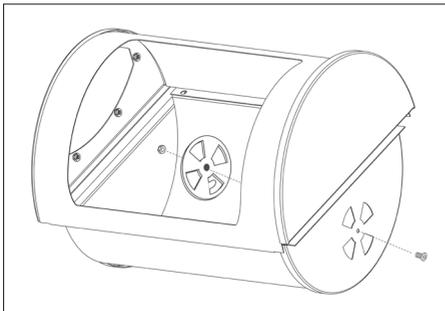
16. Mount lid stopper (25) for the small grill chamber using one M6 x 12mm bolt and one M6 nut.
