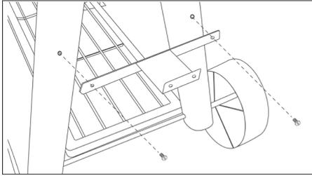
14. Connect lower part (11) and upper part (12) of the small grill chamber using six M6 x 12mm bolts.
