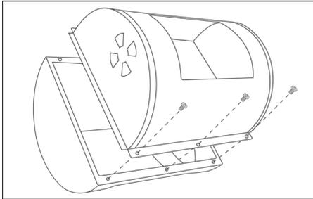
15. Mount vent slide (24) for the small grill chamber using one M6 x 12mm bolt and one M6 nut.
