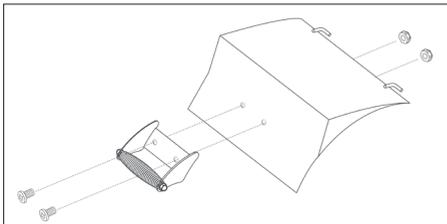
22. Attach the lids to the small and the large grill chambers. To do so, push the hinge pins through the hinges and affix them using 4 hinge bolts.
