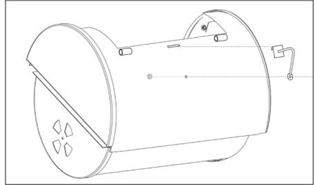
17. Attach the small grill chamber to sheet metal holder (14) and to the large grill chamber using eight M6 x 12mm bolts and two M6 nuts.
