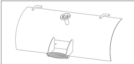
21. Connect handle (26) with the lid of the small grill chamber using the supplied 2 bolts and 2 nuts.
