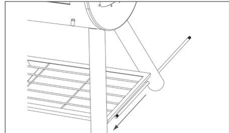
7. Fasten wheels **(6)** on the wheel axle using two M12 nuts **(B)**.
