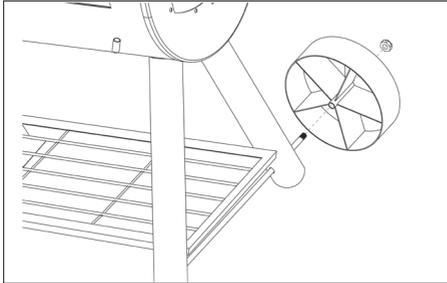
8. Place exhaust flap **(9)** over the bolt neck on the upper end of smoke pipe **(7)**. Then place spring **(8)** on the bolt neck and fasten with a cap nut.
