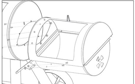
18. Attach sheet metal holder for ash collection tray (13) using six M6 x 12mm bolts and six M6 nuts. Slide ash collection tray (20) onto the rails of the sheet metal holder.
