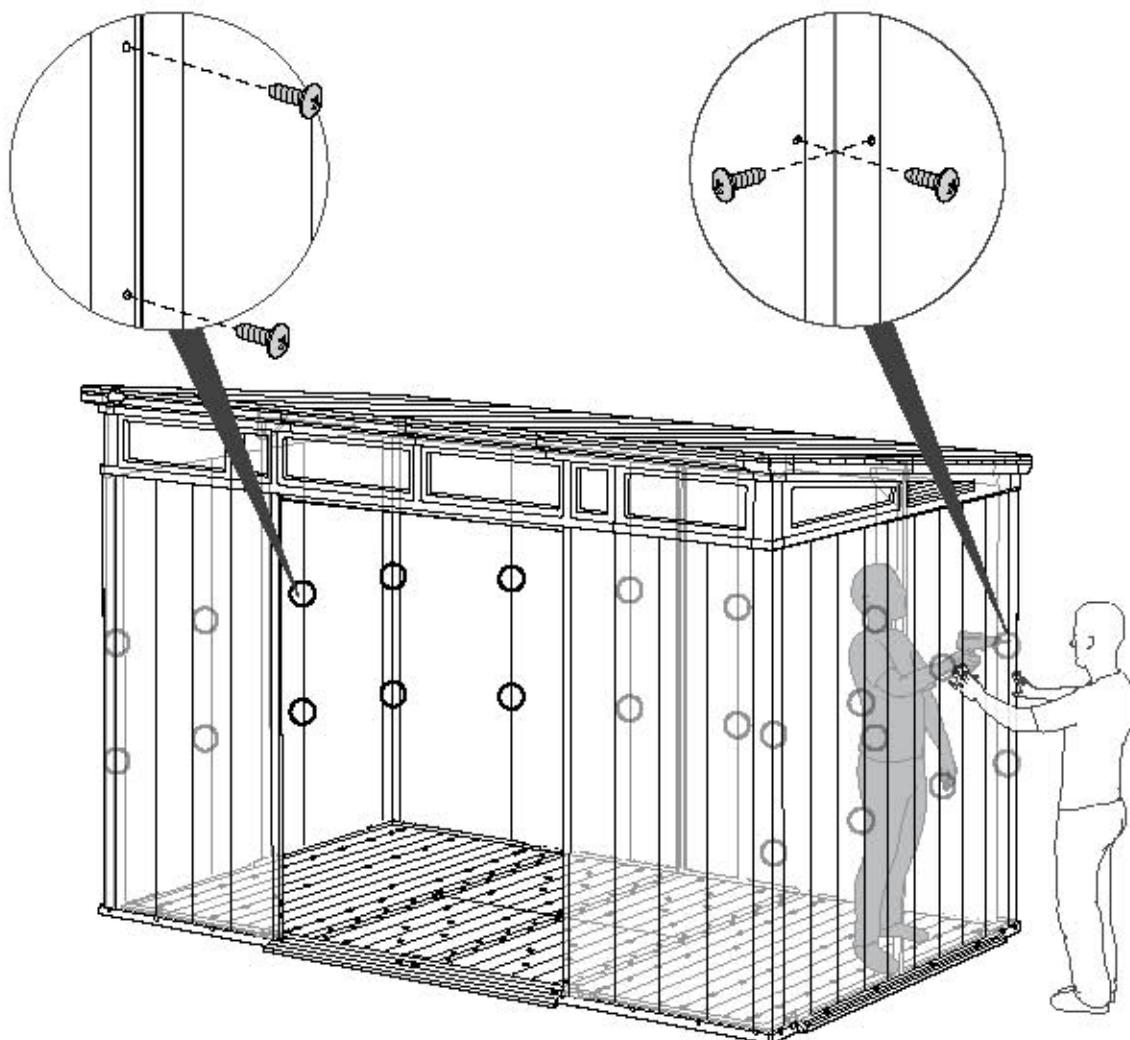
**DOOR ASSEMBLY | MONTAGE DE LA PORTE | ARMADO DE LA PUERTA | MONTAGE DER TÜR | DEURMONTAGE | MONTAGGIO DELLA PORTA | MONTAGEM DA PORTA**
