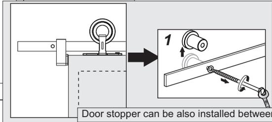
Door stopper can be also installed between two wall mounts.
