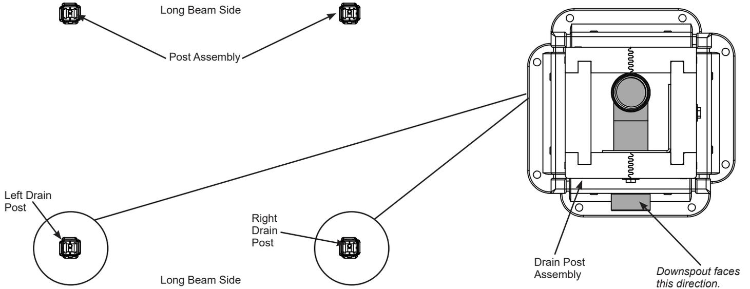
**Option 2** shows the drains downspout exiting on opposite Short Beam sides.
