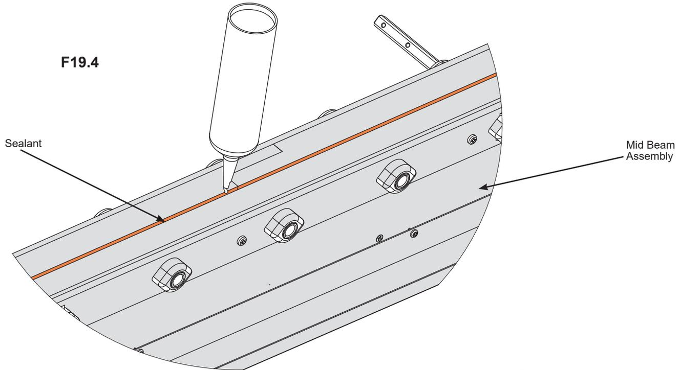
**Note:** All surfaces to be clean, dry, dust and grease free before application with temperatures above 5°C (41°F), no warmer than 35°C (95°F).
