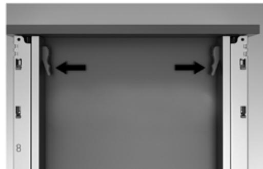
**Press the latch to the direction of the arrow to remove the drawer**
