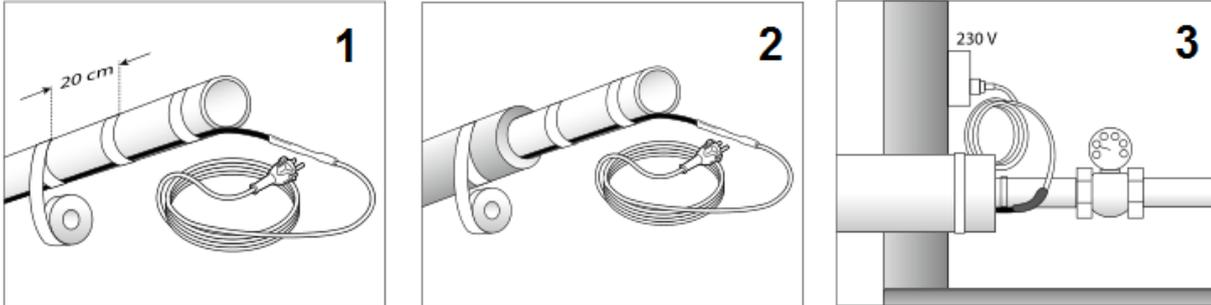
If the cable is too long, or you want greater power, the cable may also be twisted around the cable in spiral form. There is no problem the cable crosses itself, it will not overheat.
