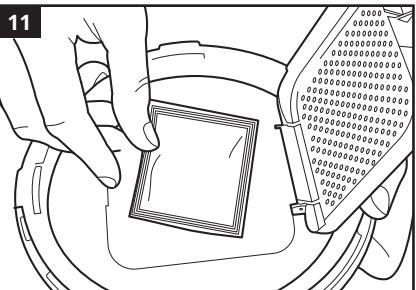
**EN** Take the desiccant pad out of its packaging and place it into the holder in the lid. Do not use the pad if it is visibly damaged.
