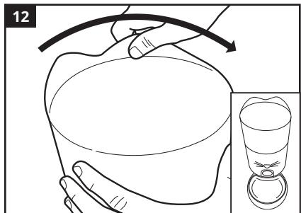
**EN** Place the lid back on and rotate it clockwise until you feel it lock into place.
