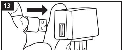
**EN** Attach the power cord to the USB adapter provided and plug it into the wall socket. Secure excess power cord with a tie wrap and place it behind the device to avoid pet chewing and entanglement of pet and/or cord.
