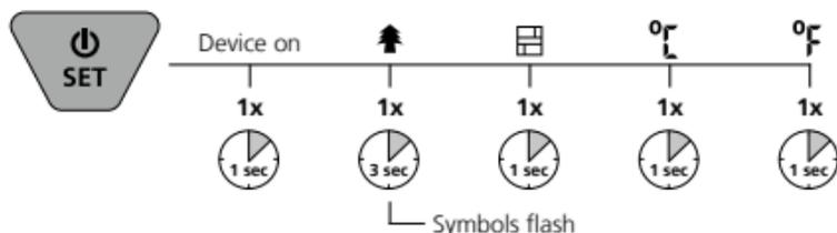
**!** The device starts with the measuring mode last selected. To select the mode, press and hold the Set button for 3 seconds or briefly wait until the symbol stops flashing.
