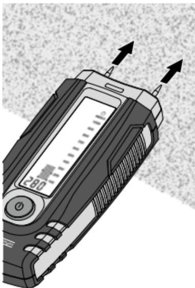
Be aware that walls (or surfaces) with differing material structures, or even variations in material composition, can cause measurement results to be falsified. Perform multiple comparative measurements.
