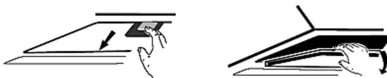
3. Plug the carbon filter into the appliance and turn in clockwise direction.
