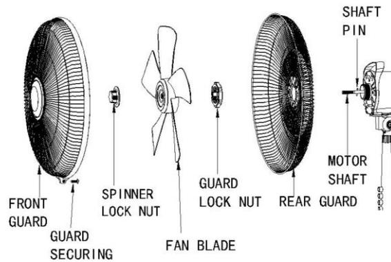
1. Remove the spinner lock nut and guard lock nut from the motor shaft.
