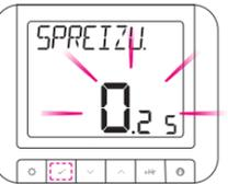
Press SELECT. Using UP or DOWN, select the Span value. Press SELECT to confirm.
