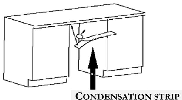
**NOTICE!** Improper installation of the condensation strip may cause damage to the worktop.
