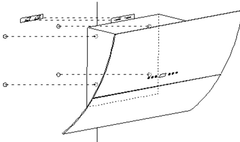
3. Hang the appliance on suspension bracket. Fix the appliance (look at step 2). The appliance must be installed in horizontal position. Check proper position using a spirit level.
