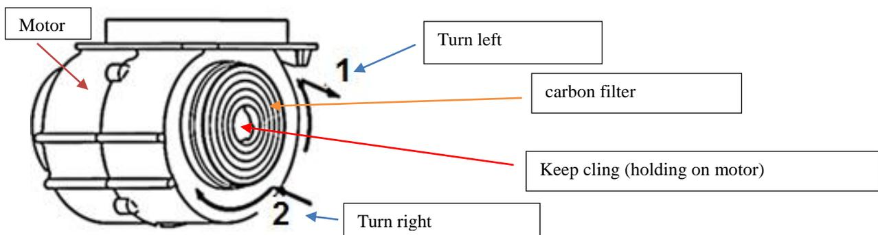
1. Turn left = The carbon filter is rotated to remove
