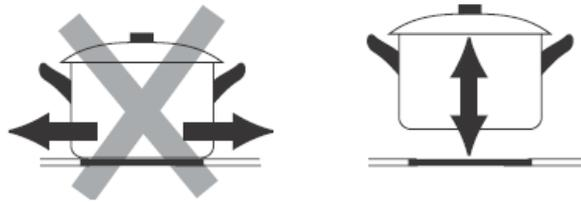
The base of cookware must have a minimum diameter relevant to the diameter of the cooking zone you use the cookware on.
