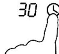
3. Set the desired time using the + and - sensor.
