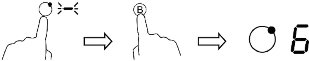
5. All cooking zones can be operated with the booster-function separately. When using the booster- function, please deactivate a running booster-function of the same group (look at chapter 3.8); otherwise p and 9 will alternately flash on the display of the selected cooking zone and power level 9 is set automatically.
