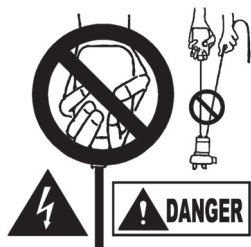
FIG. 2 Never pull the power cable or float. It may cause damage to the motor and an electric shock.
