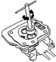
3. Install new paper gaskets, O-ring when reassembling.
