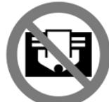
**The symbol on the device serves as a warning so that you never cover the device. Fire hazard!**
