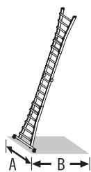
Dimensions of the setup ladder (sides extended to maximum)
