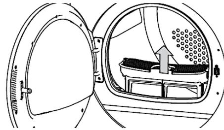
4. Open both parts of the fluff filter and remove all fluff
