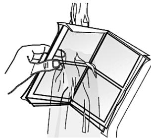
7. Insert the two-part fluff filter properly (the fluff filter **must** be dry completely).
