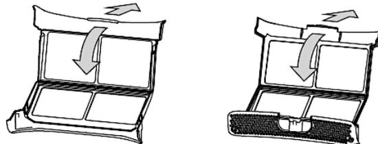
5. Clean the two-part fluff filter. Remove the residues under warm running water.
