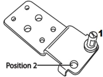
7. Fix the fixing plate with 3 screws on the opposite side. Fix the foot.
