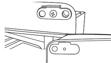
5. Tilt the appliance by max. 45° and remove the feet and the screws securing the right hand hinge plate, and the fixing plate.
