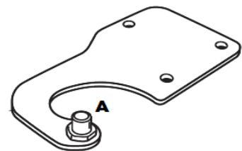
4. Remove the hinge insert plate from the bottom of the door and fix it on the opposite side.
