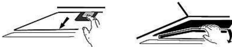
3. Plug the carbon filter into the appliance and turn in clockwise direction. Repeat on the opposite side.
