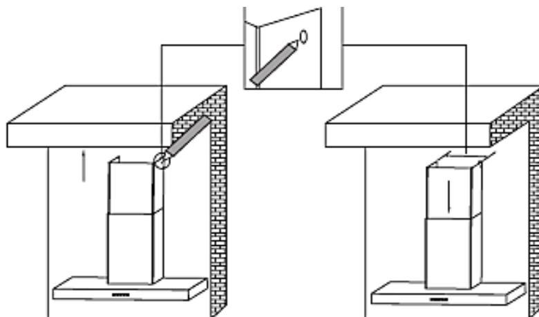
10. Drill two  $\text{\O} 8$  mm holes for the fixing bracket in the appropriate height. Install the fixing bracket on the corresponding position on the wall (s. fig. below).
