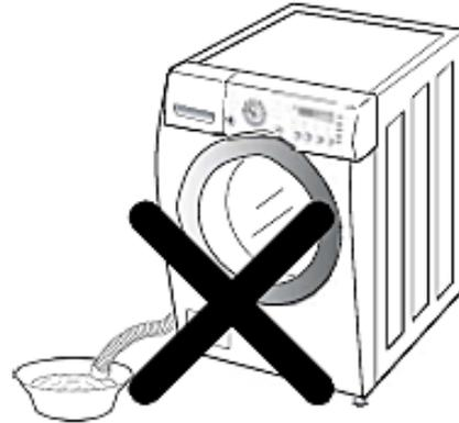
➤ The hose outlet **must not** be submerged into water.
