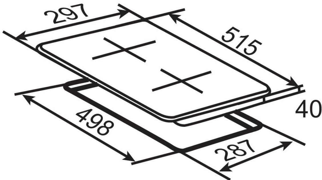
➔ The safety distance between the hob and a cupboard above should be at least 760 mm.
